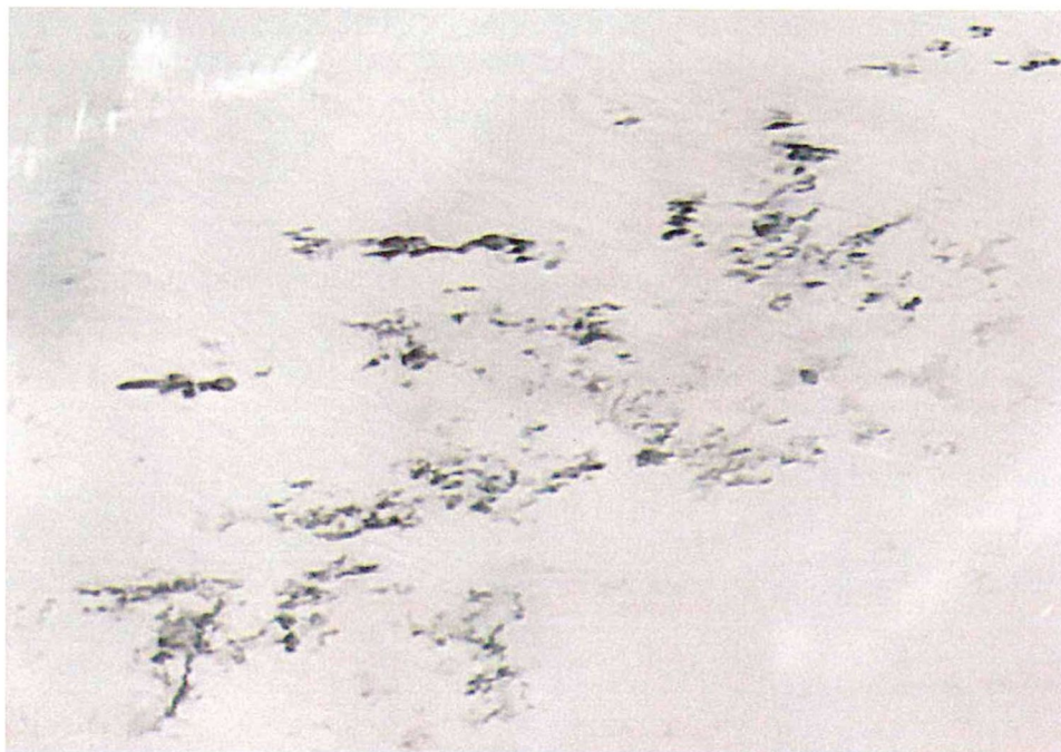
Stress Corrosion Cracking on Spar Cap
