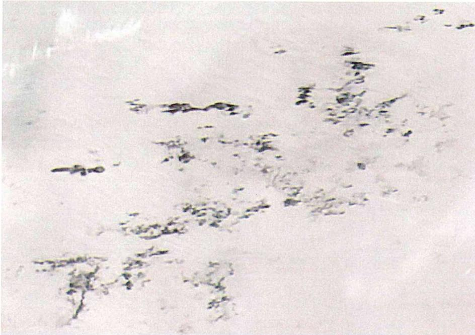
Stress Corrosion Cracking on Spar Cap
